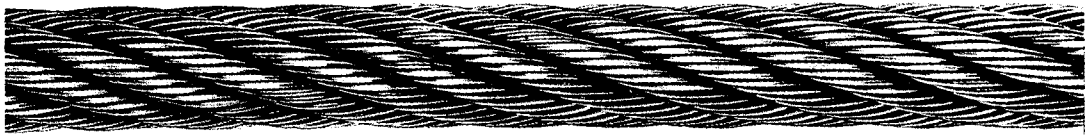
8 x 25 filler wire Type W 8 Strands, 25 Wires per Strand, 1/2 in. and larger
