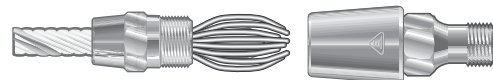
SLEEVE, PLUG & SOCKET: Plug driven in and strands closed to apply socket.
